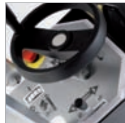
User friendly depth of cut setting and simple speed control
