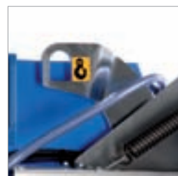
Stable, balanced transportation hook makes problem-free crane transport possible
