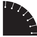
C3 Close spacing, narrow slots with keyhole
