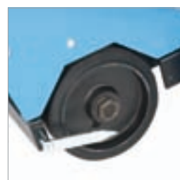
Machine is exactly aligned using cut indicator
