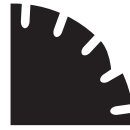
C1S Wide spacing, wide slots Oblique protective segments against undercutting effect
