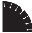
C3S Close spacing, narrow slots with keyhole Oblique protective segments against undercutting effect
