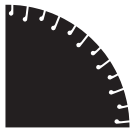
C6 Close spacing, narrow slots with keyhole
