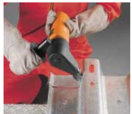
FEIN nibbler for distortion-free cutting through flat and curved sheet metals.
