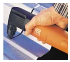
BLK 1.6 - Flexible in all Directions: Job-alignment without tools, adjustable in 45° steps up to 360°.
