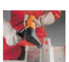
FEIN nibbler for distortion-free cutting through flat and curved sheet metals.
