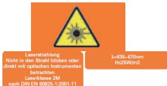
Laser class 2M warning labels on the laser instrument.
