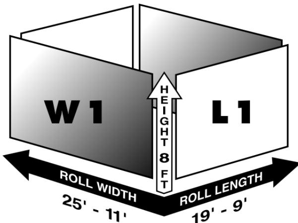
You will only need to roll a length and width, and roll or set a height. Then you can calculate the total wall surface area of that room. See the “Taking Volume Measurements” section for information on rolling or setting a fixed height.
