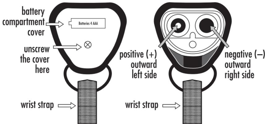
2. Remove all four batteries and insert four new ones. Insert two of the batteries on the left side with the positive ends facing outward; insert the other two batteries on the right side with the negative ends facing outward (see diagram).
