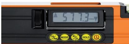
Zero calibration / Reference    Mode    Sound / Illumination    Hold    Power
