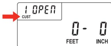
2. Press [SET] then press [SCALE] [SCALE] to begin entering the Custom Scale.
