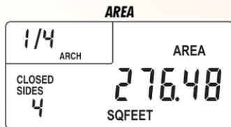
7 Press the [CLOSE+] key followed by the [SET] then [M+] keys. Now press the [MR] key to display the Adjusted Area. Press the [SET] then [MR] keys to clear the Memory.
