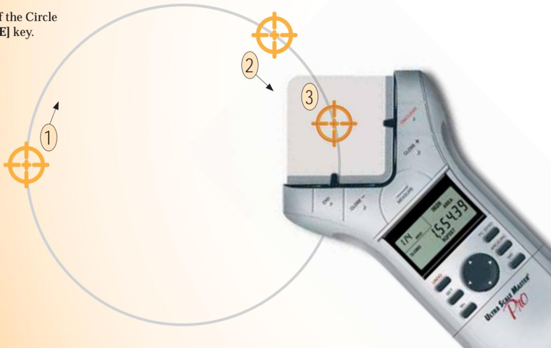
4 Upon pressing the [MEASURE] key in Step 3, the Circle measurement was automatically completed and the Circle Area displayed. Once a Circle measurement is completed, press the D-Pad down [▼] to display Circle Perimeter, Circle Wall Area, Circle Volume and stored Height. Continuous presses of the D-Pad down [▼] or up [▲] will scroll back and forth through the values.
