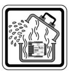
Do not store the laser when wet. Dry the laser and case before putting the laser away.
